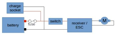
receiver, usually with built-in speed controller, batteries and motor connected as shown on the right. A switch is needed to isolate the battery when the loco is not in use and some method of connecting to a charger is also required - both can be achieved simply with micro plugs/sockets. A fuse in the battery positive lead is recommended to protect the battery in case of inadvertent shorts while working on the loco.
