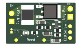
10A without a heatsink at a max of 30V. When off, MSW13a draws no current so may be permanently connected to the battery. The on-board LED can be used to provide an 'on' indication or can be connected to a Micron receiver LED2 output.
