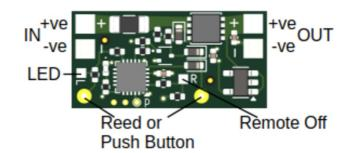
MSW11a is available as: a bare board with reed switch mounted; or without reed switch mounted (e.g. for use with a push button); and with optional input, output and charge connector wires.
